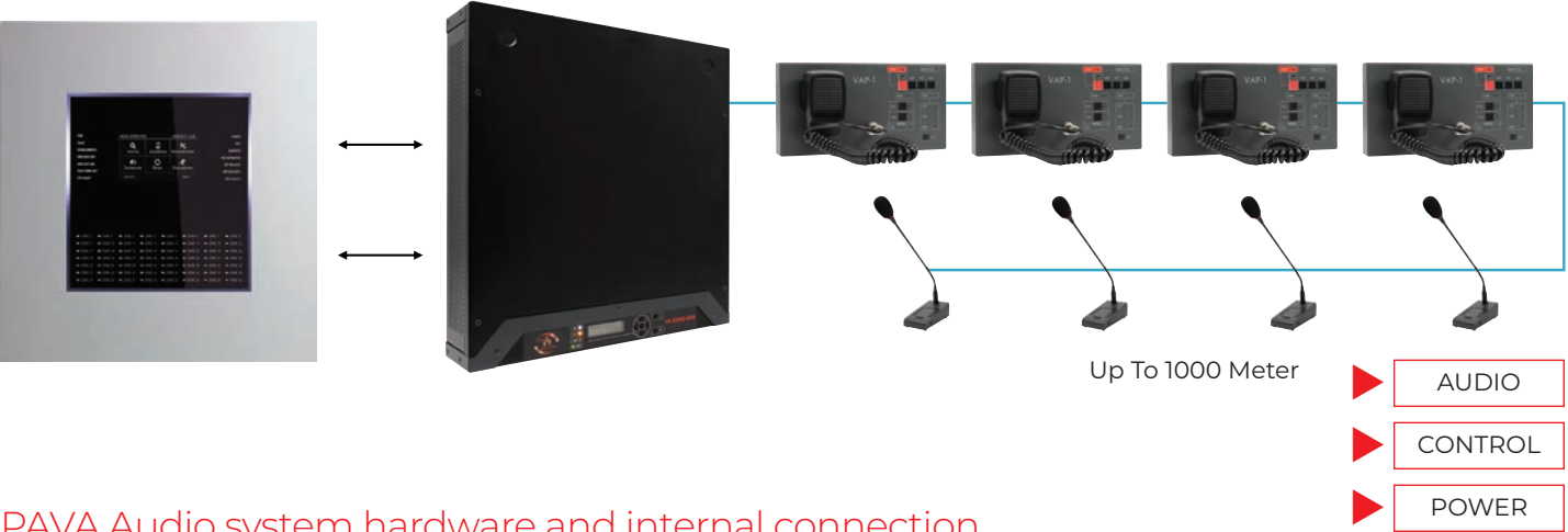
PAVA Audio system hardware and internal connection
